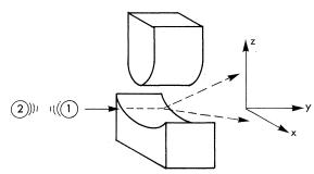
Fig. 1. Schematic illustration of the apparatus for the Einstein, Podolsky, and Rosen experiment.
