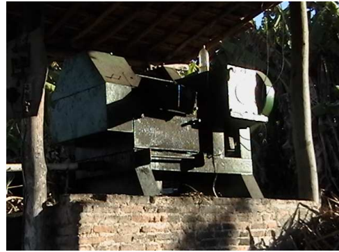
Fig. 2d. Three rolls mill.
